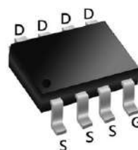
SOP8 Pin Configuration
